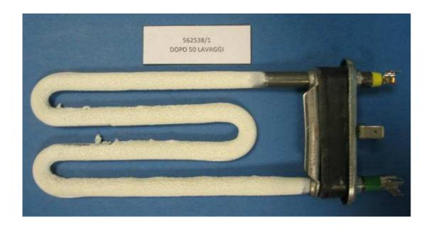
Heating element of the washing machine WITH device
